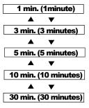
The time for the auto power off function can be specified only when using the batteries.
